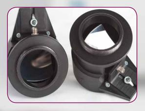
Variety of fiber probes coupling with any FTIR spectrometer
