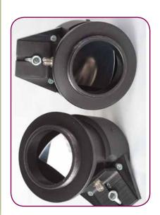
Two identical mirror couplers are designed to focus FTIRbeam to fiber probe input or refocus it from the probe output to FTIR-detector. Can be installed directly at sample chamber windows, at external FTIR port or be fixed with a customized holder inside sample chamber. Mirror optics covers a broad spectral range and can be adjusted to SMAconnector position to maximize coupling efficiency. Mirrors can rotate around beam axis for convenient probe connection to FTIR at any angle.
