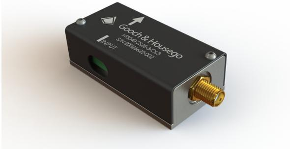
A compact Acousto-Optic Frequency Shifter featuring low power 100mW 40MHz supply requirement and high diffraction efficiency, this device is ideal for use in heterodyne interferometric systems, particularly laser Doppler velocimetry and has been designed to facilitate double pass configuration.
