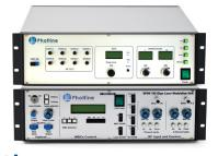
The ModBox-DQPSK and ModBox-OFDM are bench-top Modulation and Demodulation Units dedicated to digital (D)QPSK and OFDM modulation transmission and operating in the C-band.
