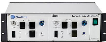
Modbox-AN-Tx and ModBox-AN-Rx are a family of turnkey optical transmitters and receivers for analog applications.
