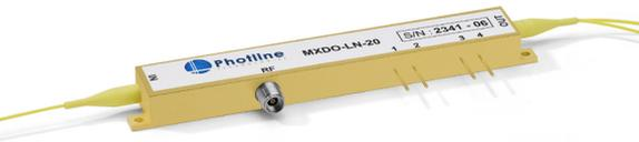
The MXDO-LN-20 is a lithium niobate (LiNbO<sub>3</sub>) intensity modulator with dual fiber outputs designed for analog applications at frequencies up to 20 GHz. The MXDO-LN-20 specific design offers an excellent balance of the two complementary fiber outputs.
