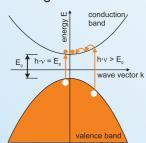
absorption of photons if E < h · v</li> => creation of electron-hole-pairs
