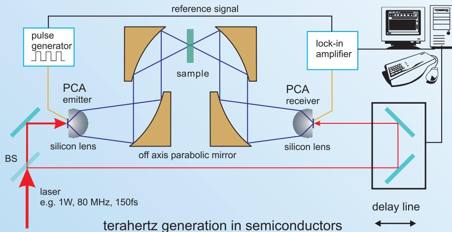
single gap photoconductive antenna - PCA
