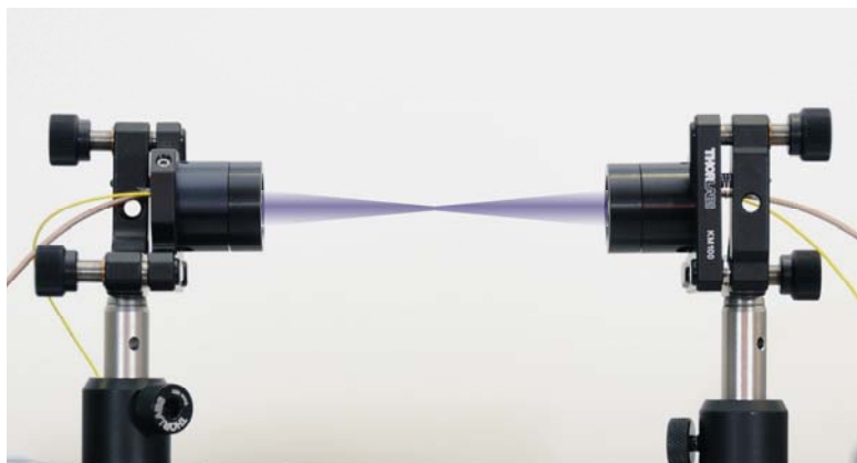
fiber coupled antennas with focusing aspheric silicon substrat lens
