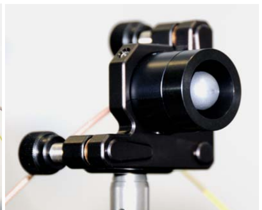
fiber coupled antennas with focusing aspheric silicon substrat lens
