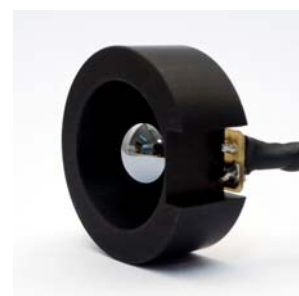
Back view with hyperhemispheric silicon lens
