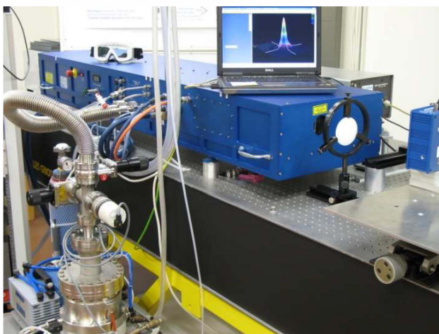
Fig. 1. The molecular gas laser with its gas handling infrastructure is the core instrument of the THz detector calibration facility. The focal beam profile at each laser line is measured by a pyroelectric THz camera.
