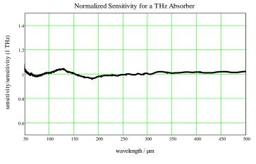
This figure shows the sensitivity of the pyroelectric detectors normalized with the sensitivity at 1 THz. Between 200 and 500 µm the sensitivity changes within 2 %.
