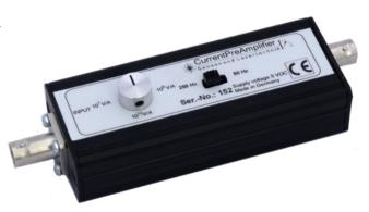
The amplification can be set by a 4-step switch: e.g.  $10^7$ ...  $10^{10}$  V/A; the bandwidth is fixed\* to e.g. 50Hz or 250 Hz. The detection limit depends on the amplification, the bandwidth and detector diameter.
