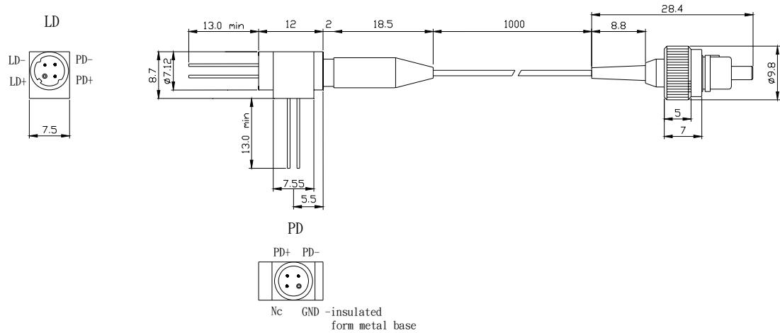
Note: The metal part is at +V (LD+). Precaution must be taken to avoid shorting the LD+ to GND.
