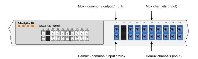
Please note, that above layout refers to a DWDM-MUX-8 Unit and is taken only as example. The actual layout of the unit described in this document depends on a number of factors such as channel number and connector type. However, the principal scheme will stay the same.
