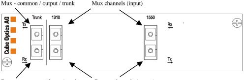
Demux - common / input / trunk Demux channels (output)
