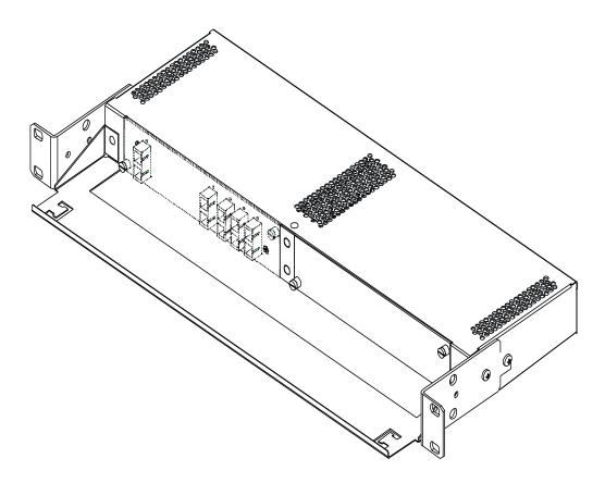
The drawing shows the Shell with 1 integrated module. The modules have to be ordered separately.
