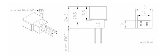
The drawing above shows the mechanical dimensions of a Raman-Filter.
