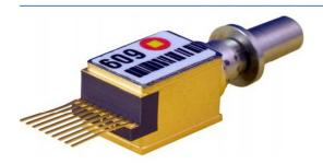
The Multiplex T510 & T51E series EML TOSA modules consists of a multi-quantum-well laser and a monolithically integrated electro-absorption (EA) modulator in a hermetically sealed metalized ceramic package. State-of-the-art, epoxy-free laser welding is utilized. The laser module also contains a thermoelectric cooler and a monitor photodiode.
