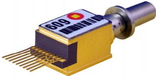
The Multiplex T510 & T51E series EML TOSA module consists of a multi-quantum-well laser and a monolithically integrated electro-absorption (EA) modulator in a hermetically sealed metalized ceramic package. State-of-the-art, epoxy-free laser welding is utilized. The laser module also contains a thermoelectric cooler and a monitor photodiode.
