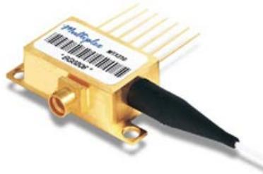
The MTX510E (EML) series is a cost-effective solution for 10 Gb/s digital optical signal transmission. The modules consist of a multi-quantum-well DFB laser device with 1550nm nominal emission wavelength and a monolithically integrated electro-absorption (EA) modulator.
