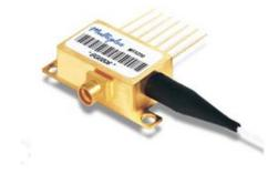
The MTX310E (EML) is a cost-effective solution for 10 Gb/s digital optical signal transmission. The MTX310E series modules are optimized to operate at a bit-rate of 10Gb/s for OC-192 and metro transmission with an excellent pedigree of reliability The very low dispersion penalty at 1310nm wavelength find wide applications over most installed intra-city optical fiber networks. The MTX310E module is well suited for reach applications up to 40km.
