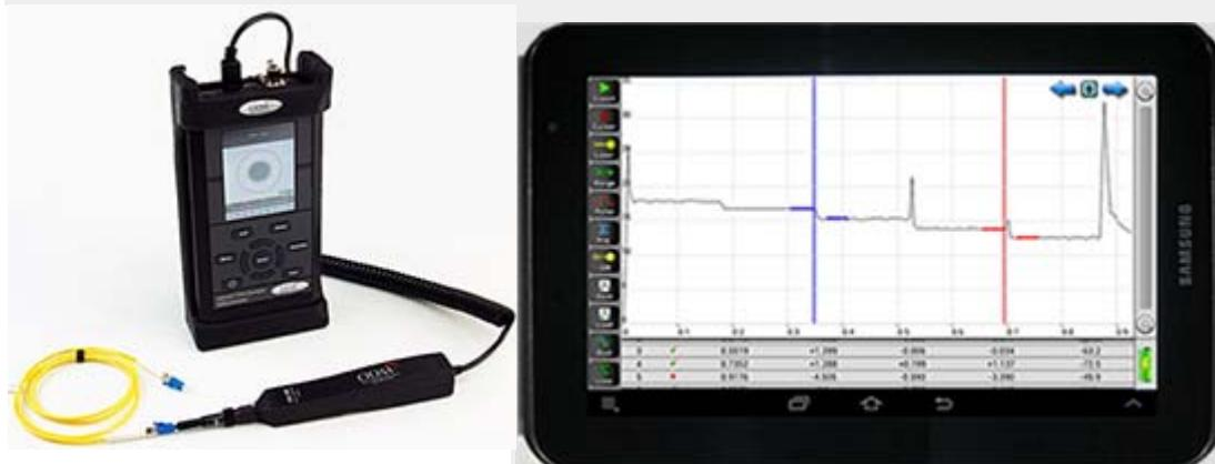
**OTR 500 with the VIS 400-HDP Inspection Scope (*left*) and an OTR Event Summary Table display on 7-inch tablet (*right*).**
