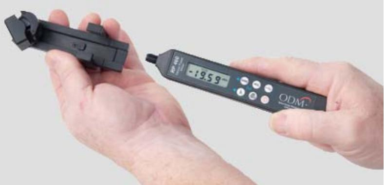
Measurements on the power meter are directly correlated to the actual core power with measurement repeatability of +/- 2dB. For more information, consult the [LFI 110 Operation Manual](#).
