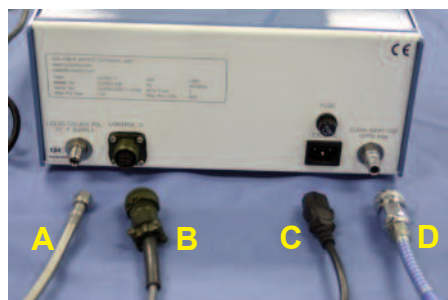
Back of the unit connections A: CO 2 connection (use 9/16" wrench). B: Foot pedal connection. C: Power connection. D: Propellant gas, Nitrogen.
