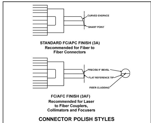
air gap between the fiber and the lens, the backreflection level for the endface of the fiber is about -14dB. This can be reduced to -40dB to -60dB by slant polishing both fiber ends to deflect the backreflected signal.
