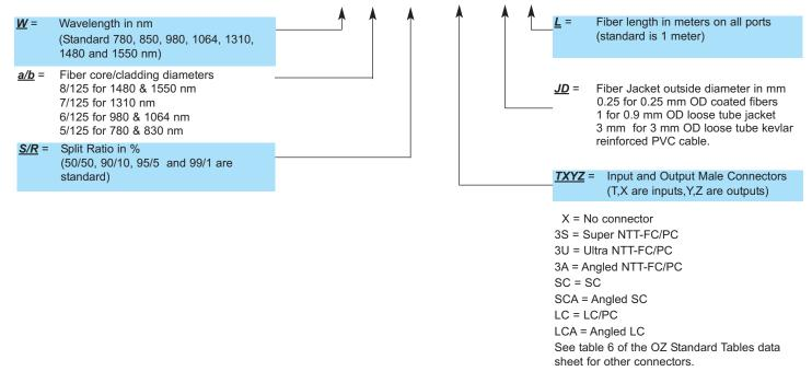
**Example:** The customer requires a singlemode two-by-two 50/50 coupler for 633nm (fiber core size is 4/125 for 633nm singlemode fiber). All ends are to be 0.5 meters long, cabled, and terminated with FC style connectors, Super PC finish. OZ Optics' part number: **FUSED-22-633-4/125-50/50-3S3S3S3-3-0.5**.
