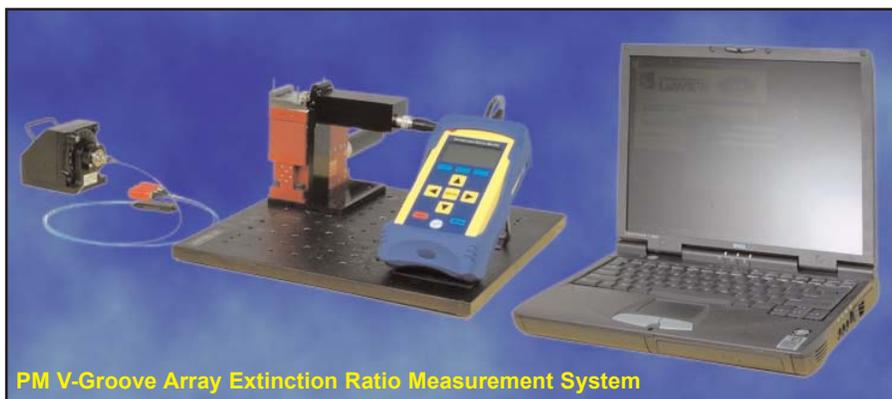
**PM V-Groove Array Extinction Ratio Measurement System**
