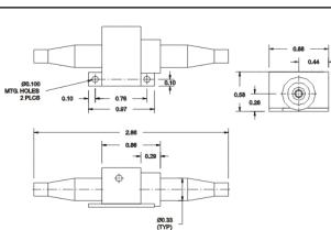
Figure 1: Neutral Density Style Attenuator Dimensions (inches)
