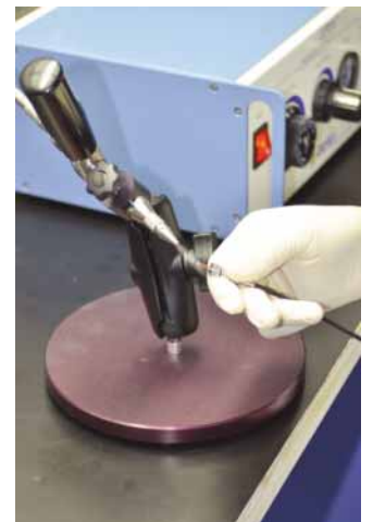
Fiber optic connector cleaning - close up.
