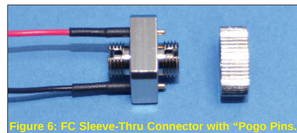
Figure 5: FC Sleeve-Thru Connector with "Pogo Pins."
