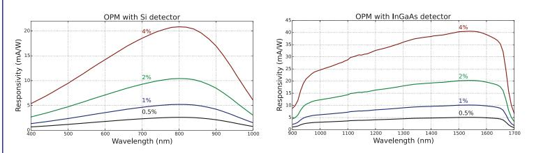
Figure 3. Responsivity of OPMs with standard tap ratios for different wavelengths
