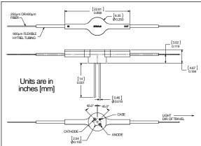
Figure 1. Dimensions of 3 PIN Optical Power Monitor
