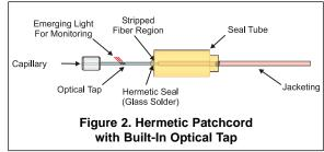
Optical taps and monitors are available in different configurations. Single channel optical taps are immediately available, either with or without photodiodes. Multiple channel power monitors for WDM applications are available upon request. Optical tap monitors are available with Si and InGaAs detectors for different wavelength ranges, while taps with Ge photodiodes are also available for a lower cost but at the expense of lower dynamic range. Please contact OZ Optics for further details.
