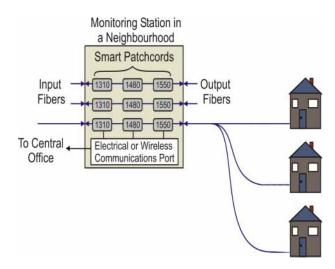
Figure 7. Remote Monitoring a WDM Network
