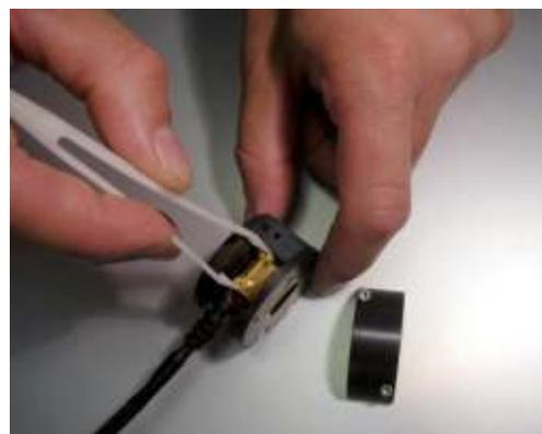
Figure 2. PPLN clip installation
